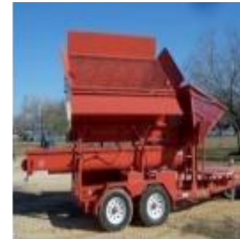
Mixing (GSM + Solidifier + Water + Soil)
